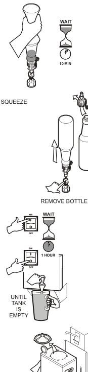
4. Squeeze solution bottle and force deliming solution into Water-Max<sup>™</sup>
